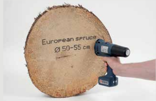
→ Cut wood printed with black universal ink (ethanol); large spacing wheels.
